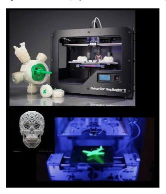
**3D printing**, or **additive manufacturing** is the process of making three dimensional solid objects from a digital model.
